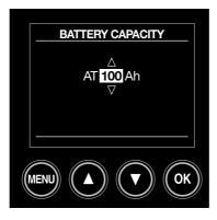
Use Up and Down buttons to change the value of battery capacity which is marked on the battery case. Press OK button to apply the changes. The default value is 100Ah.
