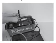
5. Use the pre-cut packaging foam to secure the battery
