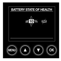
Use Up and Down buttons to change the value of low battery capacity alarm. Reduce the value to 0 to disable the alarm. Press OK button to apply the changes. The default value is 10Ah.
