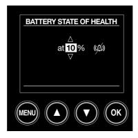
Use Up and Down buttons to change the value of battery state of health alarm. Reduce the value to 0 to disable the alarm. Press OK button to apply the changes. The default value is 30%.
