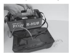
4. Secure the battery with horizontal and vertical straps provided
