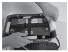
6. Connect the black battery lead to the negative terminal of the battery
