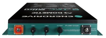
The plug shown in the leftmost photo is supplied with the battery and needs to be fitted into the "EXT RESET" port. There is a Black, Red & Yellow cable on the plug. The yellow cable stays blank while the Black and Red cable are to either end of a momentary switch. To reset the BMS you need to hold the switch while applying ≥12.8V charge voltage to the battery. **Do not hold** the switch for too long!
