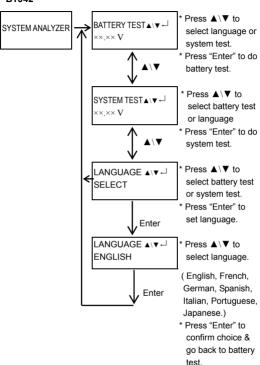
5 Press the ▲ \▼ key to select battery test. Press «ENTER» button
