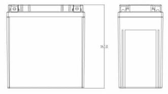
Length: 5.94in(151mm) Width: 3.43in(87mm) Height: 6.34in(161mm) Total Height: 6.34in(161mm)
