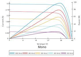
Excellent performance under weak light conditions: at an irradiation intensity of  $800W/m^2$  (AM 1.5, 25°C), 95.5% or higher of the STC efficiency( $1000W/m^2$ ) is achieved.
