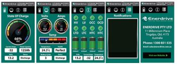
Battery Capacity, Battery Voltage, Battery Current (Amps), Battery State of Charge (SOC), Battery State of Health (SOH), Battery Status, Individual Cell Voltage, Battery Temperature, Battery Cycles, Battery Alarms & Battery Event Information.
