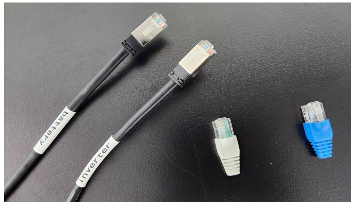
Fig. 2 - (L to R): Communication cable, Coding Terminator (grey), CAN Terminator (blue)
